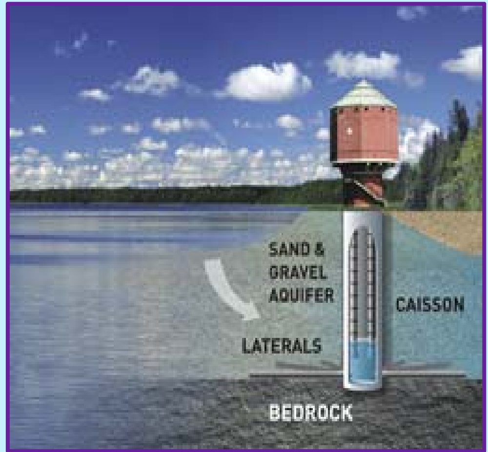
Ranney Well Collector system
