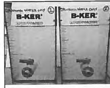
Photo 16: Jars 1 and 2 end of setting phase (30 min)
