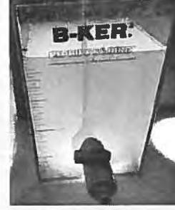
Photo 9: Jar 5 end of floc stage 3 (20 RPM)
