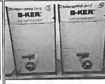
Photo 17: Jars 3 and 4 end of setting phase (30 min)
